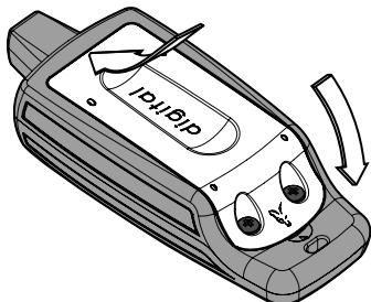
3. Take care removing the batteries. Insert new batteries and ensure correct polarity.
