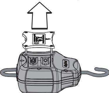
4. Take care removing the batteries. Insert new batteries and ensure correct polarity.
