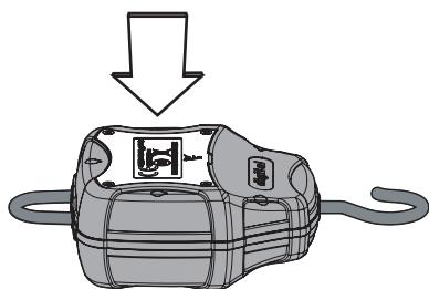
**⚠ DO NOT over tighten the battery compartment screws, excessive force will damage the screw threads.**
