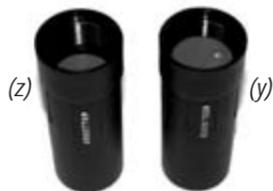
If the capsule has been fired the (red) plunger will have moved closer to the mouth of the capsule as indicated (y), the capsule is no longer effective and **MUST NOT** be screwed onto the firing head. If it is used in this condition, it will activate the firing head and inflate the lifejacket. Please Note: You will find an expiry date on the side of the capsule if this has expired **DO NOT USE**.
